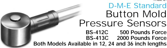
**D-M-E Button Mold Pressure Sensors** are used for measuring pressures in conjunction with auxiliary recording and control equipment in injection, die cast and transfer molds. They provide a full-scale output of 2 millivolts per volt of excitation.
